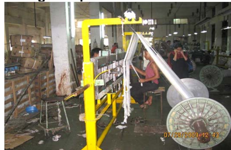
(2) Drawing the warp beam ready for weaving
