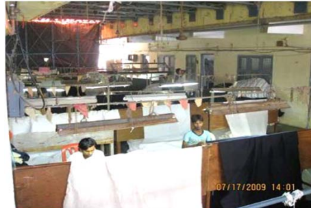
Workers spread out cloth to spot defects
