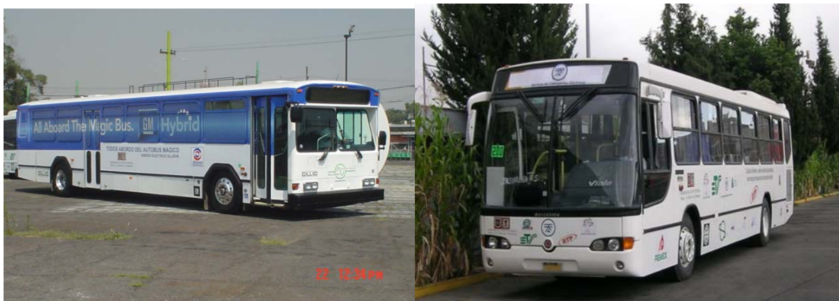
Figure 16. Parallel and series drive hybrid buses participating in the field test (Allison and Eletrabus)
