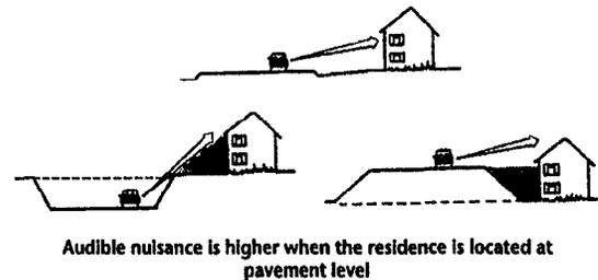
on a flat plain, because noise is reflected off valley walls. By the same token, hills and knolls can act as natural barriers to noise if they occur between the road and receptors. Above-grade roads, which are often necessary in flood-prone areas, tend to broadcast noise over greater distances.
